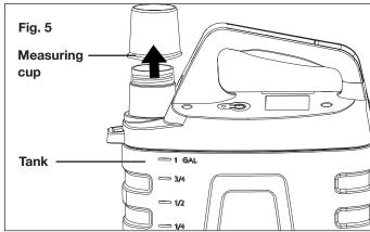
3. Fill the tank with the desired amount of water (up to 1 gallon).
